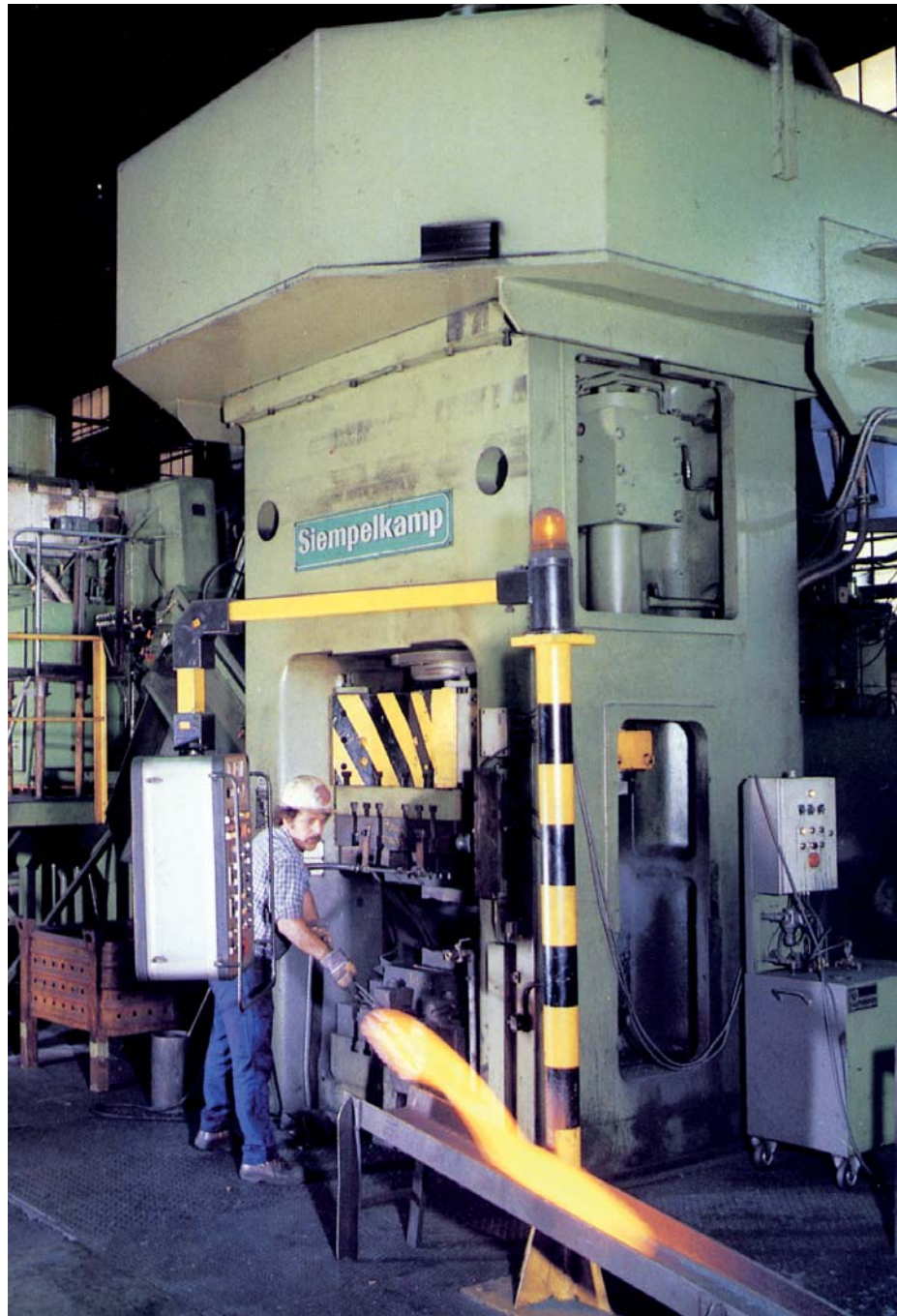
16 MN original clutch-controlled screw press
