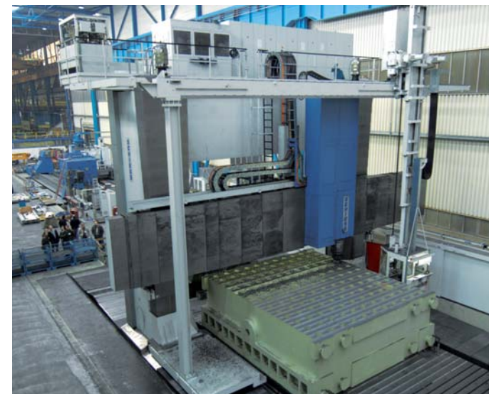
Portal milling machine machining the upper beam
