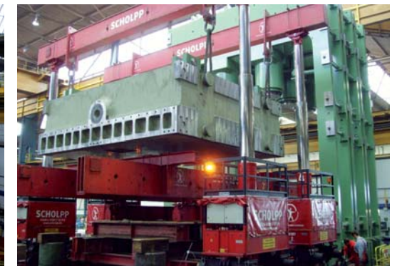
The upper beam goes into the press
