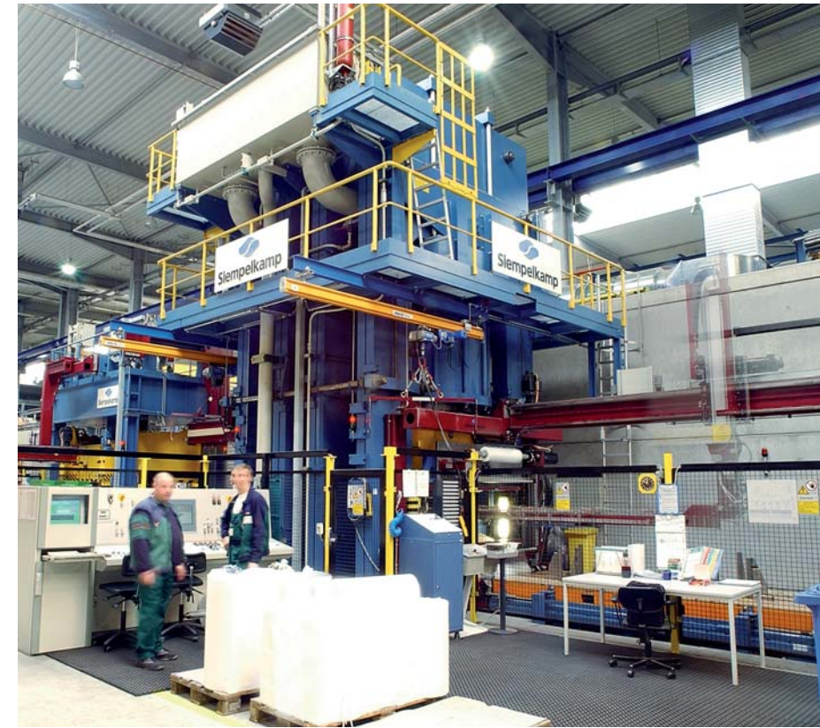
Heat exchanger plate press line, 150 MN
