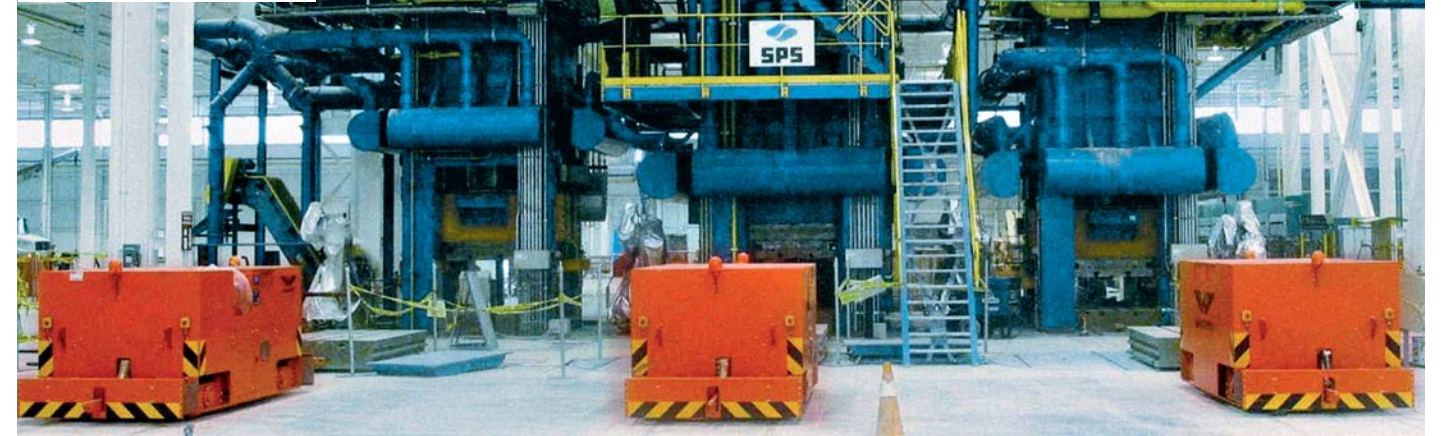
Wheel forging line, 80/50/30 MN including die-changing devices
