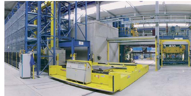
High rack stacker with fully automatic shelf stacker
