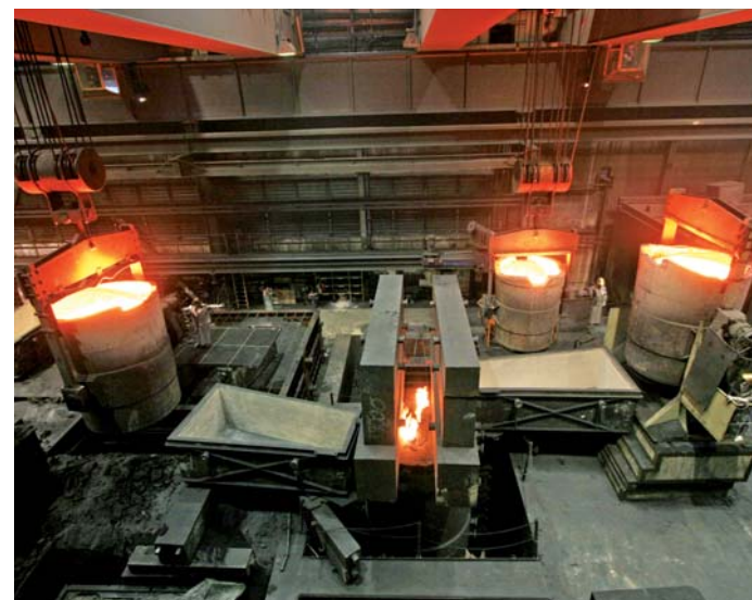
Casting of a 260 t upper beam
